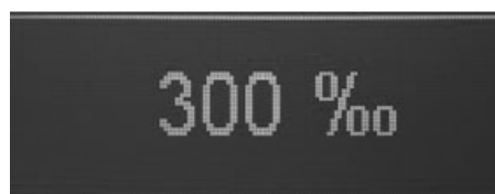
Fig.5: display of the current set point with the current measuring function deactivated
